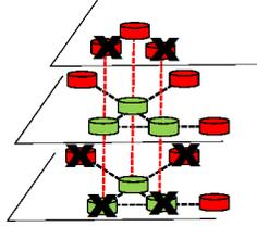
Fig. 6. A fatal sextuple failure resulting from the simultaneous failure of two data disks sharing a common parity stripe, the two parity disks of their other parity stripes and their two vertical parity disks.
