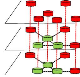
Fig. 8. A very small three-dimensional organization using six vertical parity blocks (on top) to provide expanded protection to two two-dimensional RAID arrays (middle and bottom layer).
