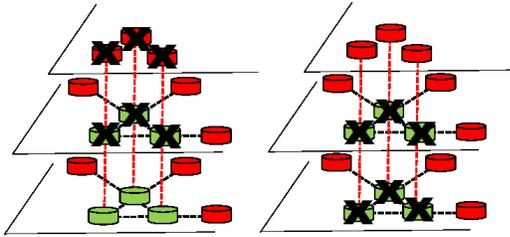
Fig.7. Two fatal sextuple failures caused by type B failures.
