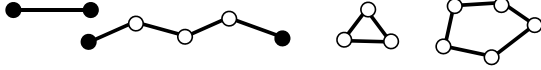
Fig. 2. Minimal irreducible failure patterns. (Failed parity disks (vertices) are represented by filled circles, good parity disks by non-filled circles, and failed data disks (edges) by lines).
