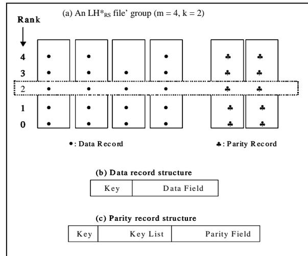
Figure 1: LH\*<sub>RS</sub> file Structure
